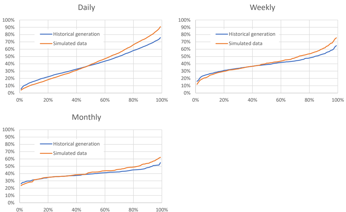
Figure 33 Daily, Weekly and Monthly comparison of simulated data with real composite data
