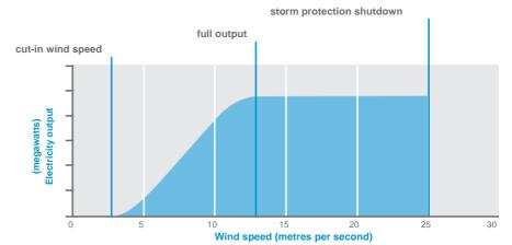
or a strong gale). At this point the turbine will automatically shut down to prevent damage.
